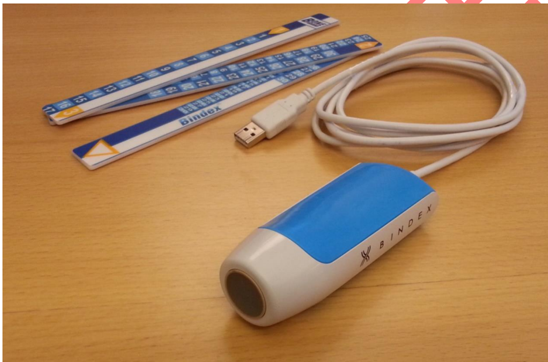
Figure 2: Bindex® BI-2 device shown together with the BI-41 Measure.
