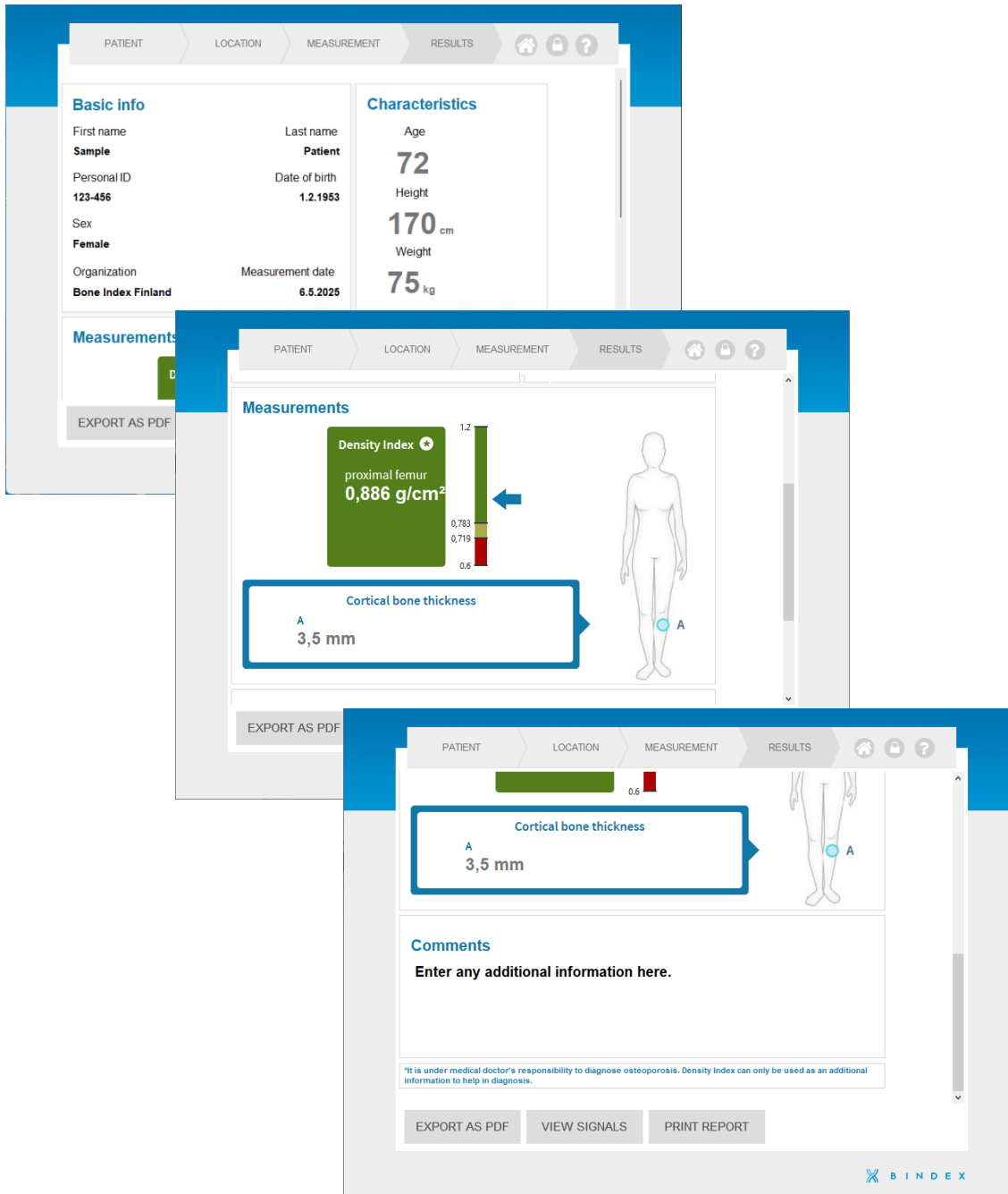
Figure 62: The result page includes patient information, Density Index and apparent cortical bone thickness values. In addition, the Density Index value is also presented on a three-color scale (green, yellow and red).
